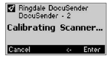
If the scanner was just powered up, the DocuSender will calibrate the scanner and report **Calibrating Scanner...** This takes about 30 seconds
