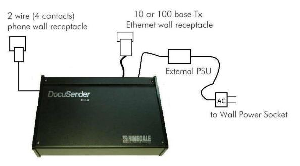
Insert your Ethernet RJ45 connection into the LAN jack.
