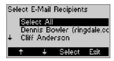
Using the arrow keys to highlight the recipient or Select All, and then press the button below **Select**. It will put an \* next to the user(s) to send e-mail to. Alternatively you can select the **Exit** option, to enter the email address manually or select "**Last**" to bring up the last email address that was manually entered. When the e-mail address sent to comes up, you can take the <- option to select the previous e-mail addresses manually entered.
