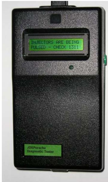
The injectors are cycled on an off on a continuous basis, until stopped by pressing enter. They are pulsed at a rate of approximately once a second, and will be heard to gently “click” each time. All 8 injectors are triggered simultaneously. This enables checks to be made to determine if one injector is not operating, and if not then the actuating voltage feed can also be checked.
