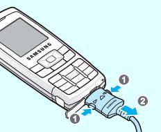
**Note:** Do not remove the battery from the phone without unplugging the adapter first. Otherwise, the phone may be damaged.
