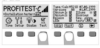
The self-test is started from the main menu with the Test kev. The test has a duration of several minutes.
