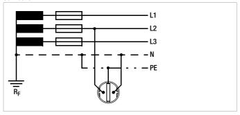
Measurement of loop impedance must be performed from all three phases (L1, L2 and L3) to the protective conductor PE for 3-phase systems in order to assure flawless functioning of the overcurrent protective device.
