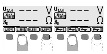
Select the limit value for allowable contact voltage, U<sub>L</sub>50VS or U<sub>L</sub>25VS, in the respective TYPE sub-menu.
