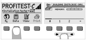
Acknowledge with the START key (press at center). All data from the selected memory address are deleted.
