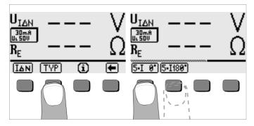
Time to trip is measured with 5 times nominal residual current.
