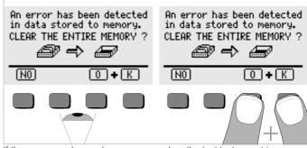
If the message shown above appears when the test instrument is switched on, you are provided with the opportunity of uploading and saving all data to a PC before deleting the memory in order to correct the error.
