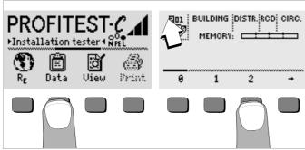
First create the desired memory address with the help of the softkeys. After acknowledging with the START key (press at center), the cursor appears at the first data entry position (BUILDING).
