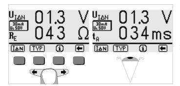
Press the start **START** key in order to measure U<sub>IANI</sub>, and continue to hold it depressed even after the measurement value has been displayed. The trip test is started automatically after contact voltage U<sub>IAN</sub> has been measured.
