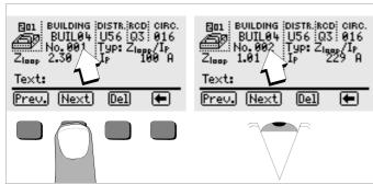
If you discover that a measurement value for the currently selected electrical circuit is missing, the required measurement can be performed immediately.
