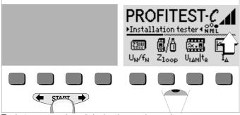
The instrument can be switched on by pressing any key.
