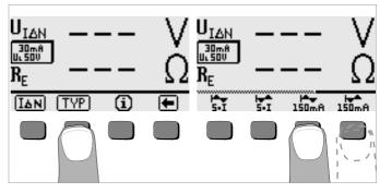
Time to trip is measured with a 150 mA constant current.
