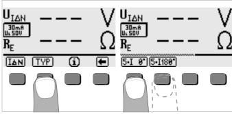
Then select 5-1 — in the TYPE sub-menu and perform the trip test with the positive half-wave.
