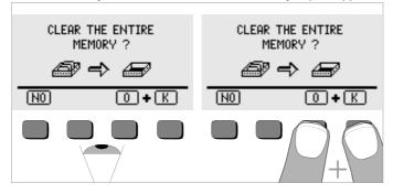
Acknowledge by simultaneously pressing O and K to delete all data from memory. The indicator to the right of the "SPEICHER:" parameter appears empty. Memory address "001" is displayed at the left. New data can now be entered for this address, or the database can be exited (press \( \triangle \) or **START** 9 times).
