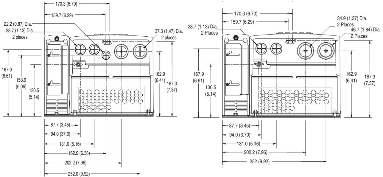
*Dimensions are in millimeters and (inches)*
