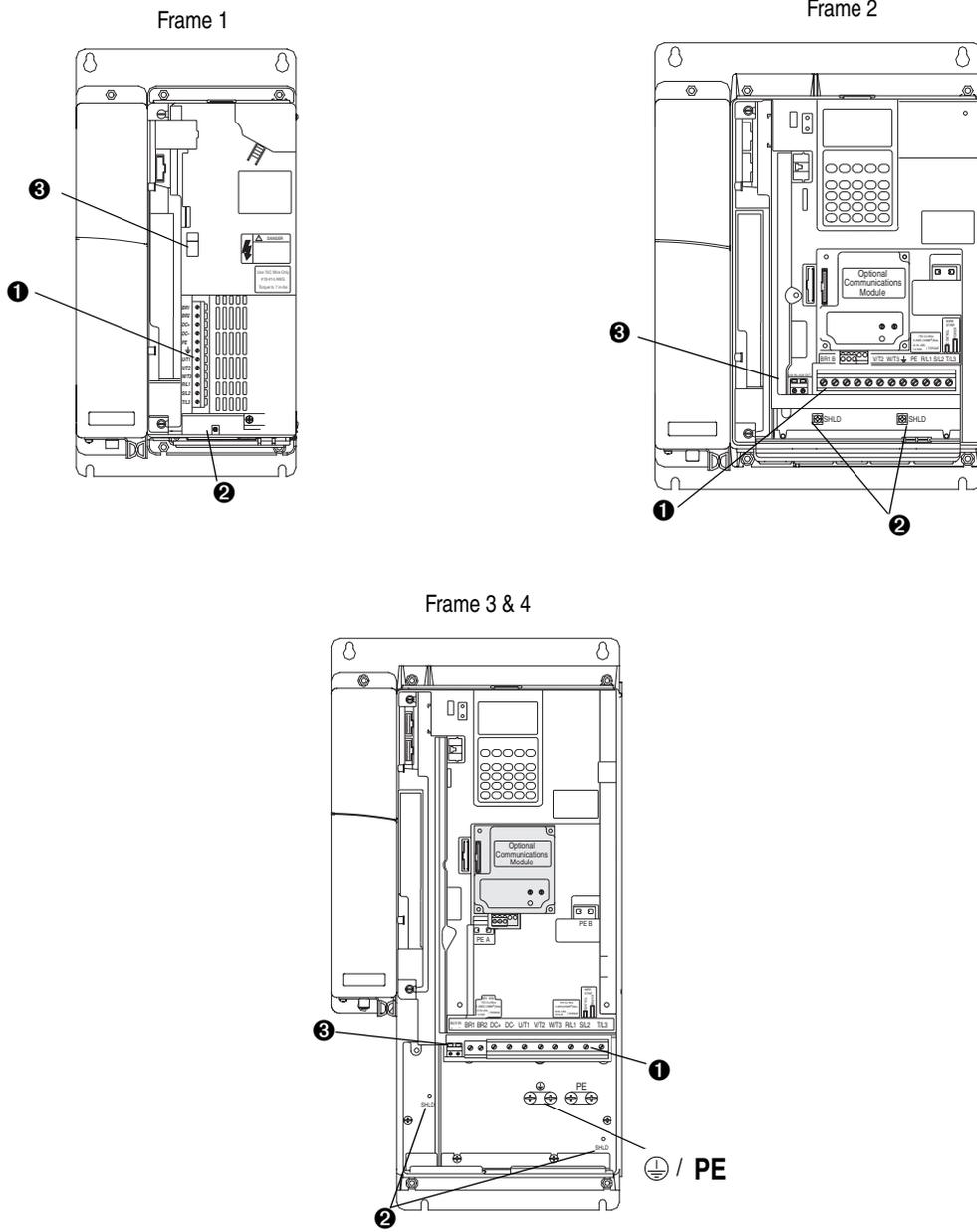
Figure 8 Power Terminal Block Location, Cont'd
