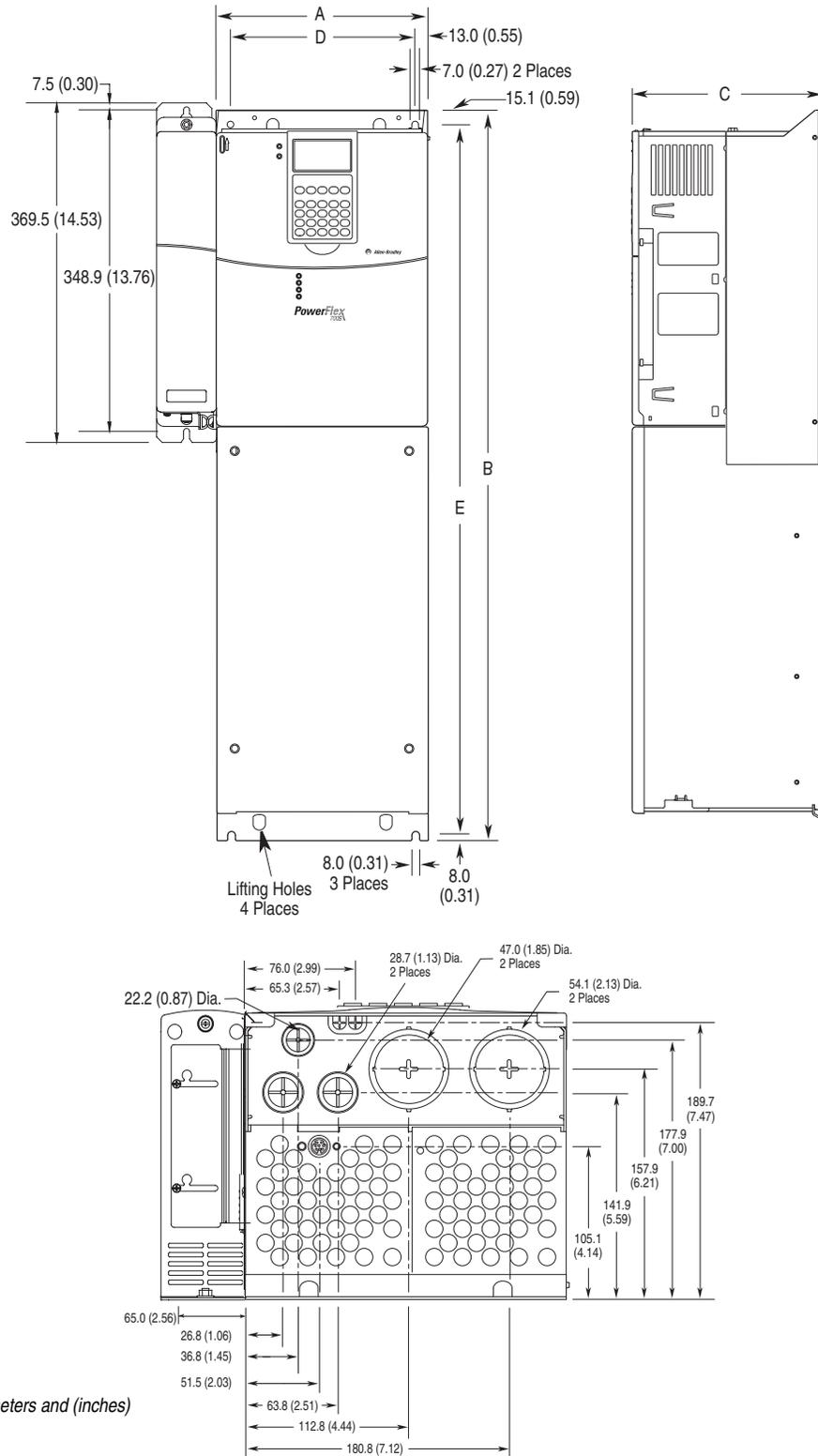
Dimensions are in millimeters and (inches)
