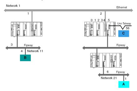
In the first case, station B addresses station A's system:
