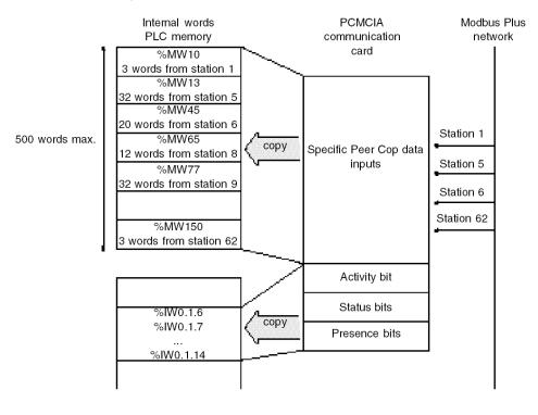
In the following example, the address of the first internal word is %MW10:
