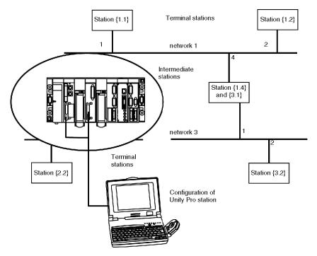
**NOTE:** Multi-network routing information is constructed at the station level at the time of configuration of each bridge. No consistency check is done on routing data for the same network architecture.
