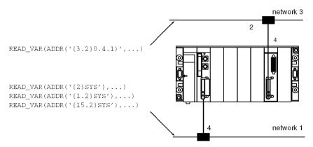
All messages intended for network 3 are sent to the coupler with module address 4, and those whose destination network is 1 to the network link integrated into the processor.
