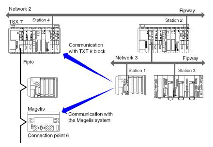
The address of the TXT 8 text block on the TSX 7 PLC station 4 is:
