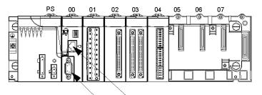
Rack 0. Module 0. Channel 3: Ethernet port (available on BMX P34 2020/2030/20302 processors)
