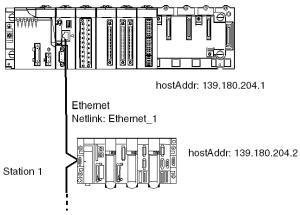
Address settings station 1: ADDM(`0.0.3{139.180.204.2}') or Address settings station 1: ADDM(`Ethernet\_1{139.180.204.2}')
