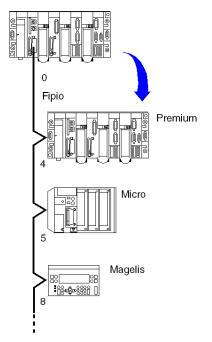
Address settings of device 4: ADDR ('\2.4\SYS') Address settings of device 8: ADDR ('\2.8\SYS')
