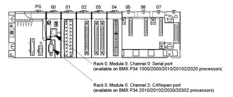
The diagram below shows an example of Modicon M340 configuration including a BMX P34 2030 processor and the addresses of the processor communication channels:
