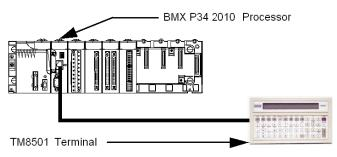
The address settings of the TM8501 terminal are ADDM ('0.0.0') or ADDM ('0.0.0.SYS').
