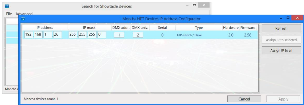
Setting the Moncha.NET IP, DMX and Universe
