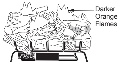
Figure 26 - Incorrect Burner Flame Pattern
