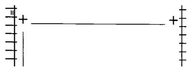
Figure 3-6. Control Crosses centred between Ticks on Guide.
