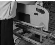
NOTE: The mounting brackets on the head/foot board should have the push/pull bar facing away from the bed.
