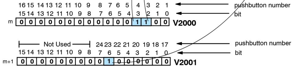
**Controlling LEDs Separately with the DL250/350/450**
