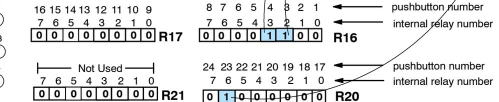
**Note:** To determine the control relay number, use the register number as the first two digits and the bit number as the last digit. For example, Bit 3 of R16 is referenced as C163.
