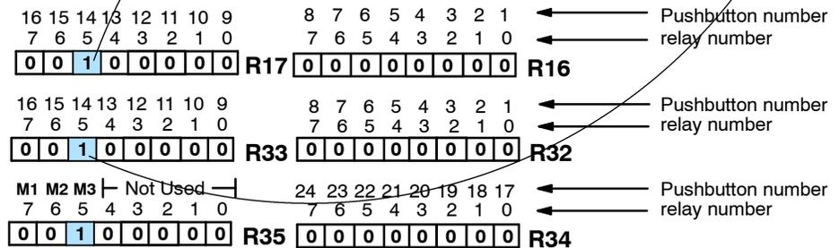
**Note:** To determine the control relay number, use the register number as the first two digits and the bit number as the last digit. For example, Bit 5 of R33 is referenced as C335.
