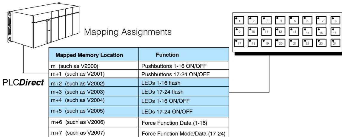
**How the Memory is Used-**Looking at the above memory map, **m+6** stores the forcing data for Pushbuttons 1-16 and **m+7** stores forcing data for Pushbuttons 17-24. There are three modes of the force function. These modes are controlled by the 3 most significant bits of m+7.
