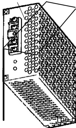
A two-prong male connector is on the rear of the unit. Your OP-panel is shipped with the female connector.
