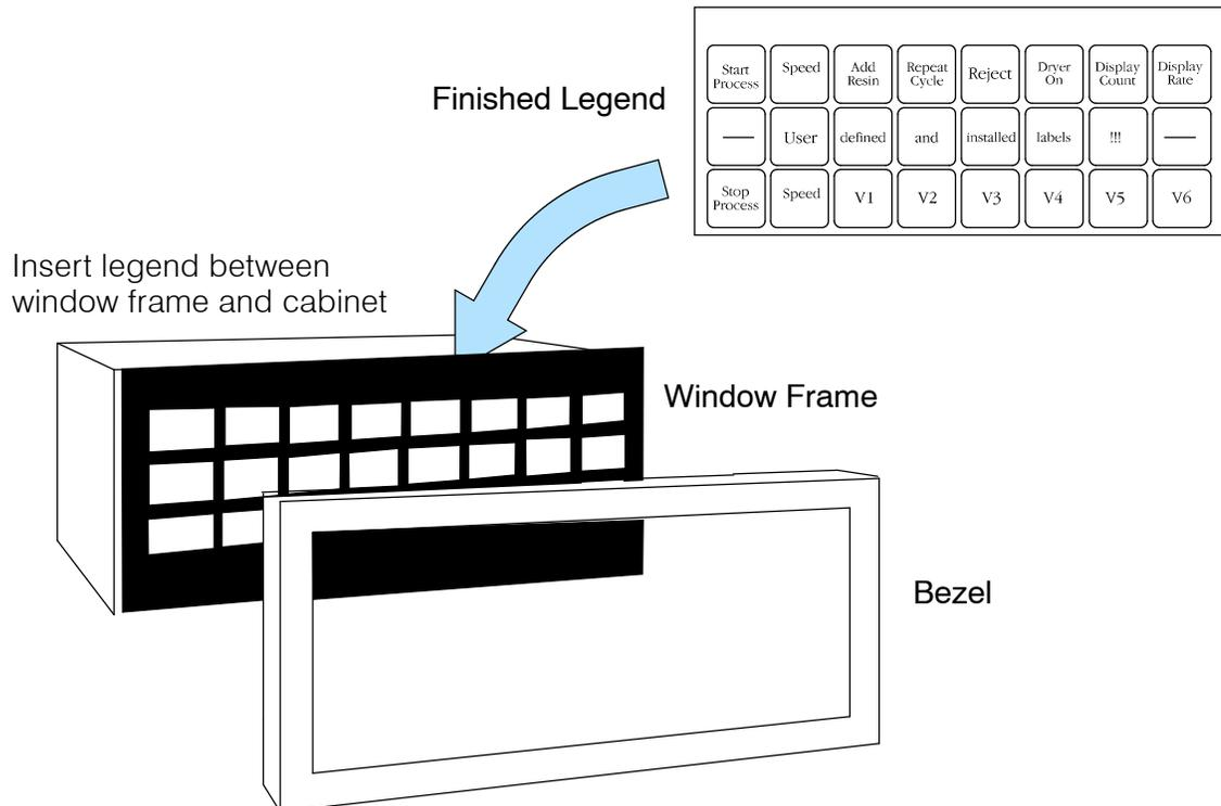
3. Slide the finished legend into the pocket space between the window frame and LED bars.
