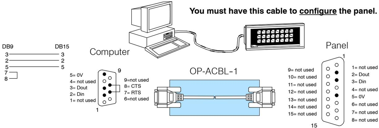
**PLC to Panel Cable** The OP-ACBL-1 (shown above) is also used to connect Allen-Bradley SLC 5/03 and 5/04 PLCs to an OP-1224 panel. Since the OP-1224 is compatible with all of the **PLCDirect** and compatible CPUs, your cabling requirements will vary depending on the CPU type you are using. Refer to the table on the next page for matching the proper cable to your PLC. Pin diagrams refer to the ends of the cables and not the communication ports.
