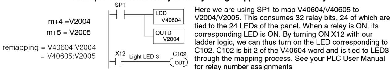
**Using Pushbutton Status Via Ladder Logic**
