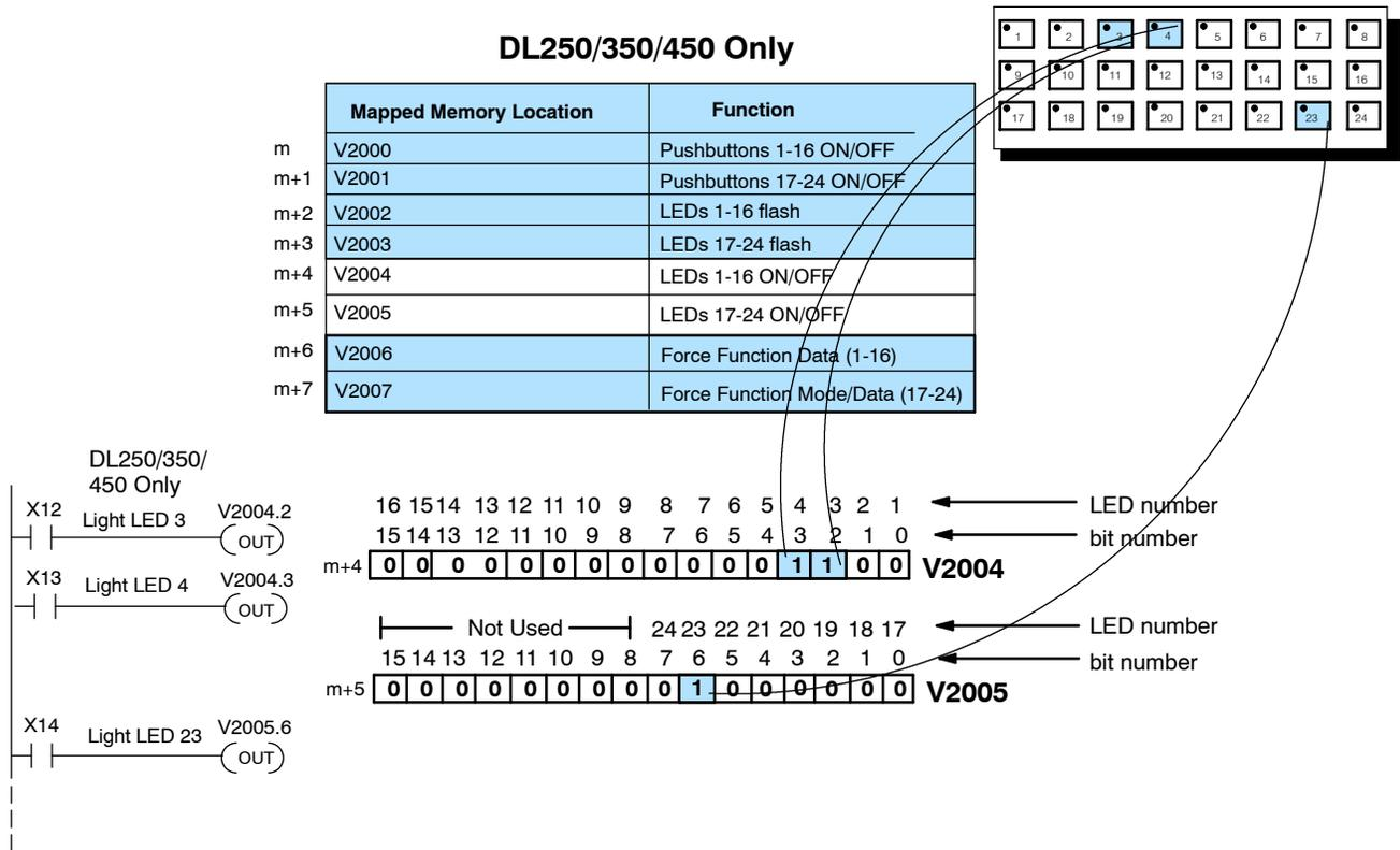
**Adding Flashing with the DL250/350/450** If you plan to use this feature with one or more pushbuttons, there are three things you must always remember during configuration:
