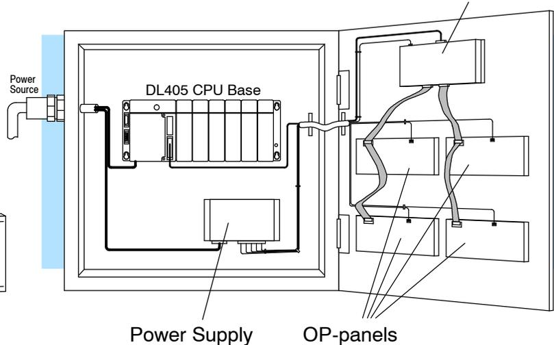
**NOTE:** Please read and follow the cabling requirements in the OP-9001 User Manual (OP-9001-M) when using multiple panels. Failure to follow the guidelines of the User Manual may affect the integrity of the RS422 link, resulting in communication errors.
