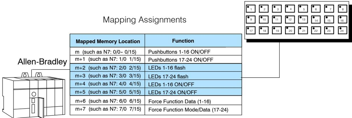
**How the Memory is Used-**Looking at the above memory map, **m+6** stores the forcing data for Pushbuttons 1-16 and **m+7** stores forcing data for Pushbuttons 17-24. There are three modes of the force function. These modes are controlled by the most significant bits of m+7.
