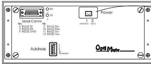
You must use an external power supply that can deliver voltages in the 8 to 30 VDC range, and can supply 4 watts of power.
