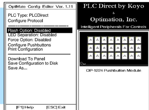
If you want to change the flashing option, position the cursor on **Flash Option: Disabled** (shown above) and then press the <Enter> key. The new screen (shown to the right) gives you a choice of **Enabled** or **Disabled**. Make your selection and press the <Enter> key again. This will return you to the original screen (top). **Note: The flash option will only work for those buttons you have configured to act as "momentary". See Step 11.**
