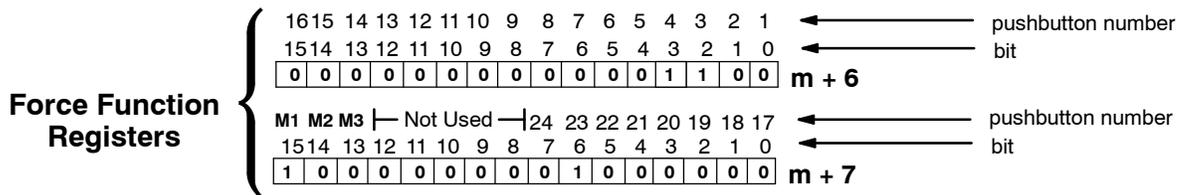
Think of forcing as a one-shot process. That is, once you have set the mode in m+7, the bit patterns in m and m+1 are changed (according to the mode selected), and then, all of the bits in m+6 and m+7 are set to zero. What this means is that all pushbuttons return to normal manual operation after the forcing is completed.
