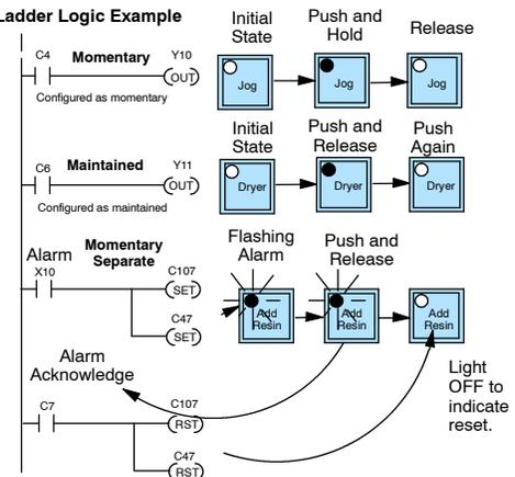
Notice in this example we are using Pushbuttons 5, 7 and 8. These are controlled by internal relays C4, C6, and C7. Your configuration software (OPEditor) allows you to operate your pushbuttons as either momentary switches or "maintained" alternate action switches. We have made C4 a momentary switch and C6 is a maintained switch. C7 is a momentary switch but we are controlling the separate ON/OFF and flashing of Pushbutton 8 with C47 and C107 respectively.
