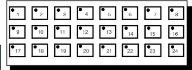
**How the Memory is Used**-Looking at the above memory map, **m+6** stores the forcing data for Pushbuttons 1-16 and **m+7** stores forcing data for Pushbuttons 17-24. There are three modes of the force function. These modes are controlled by the 3 most significant bits of m+7.
