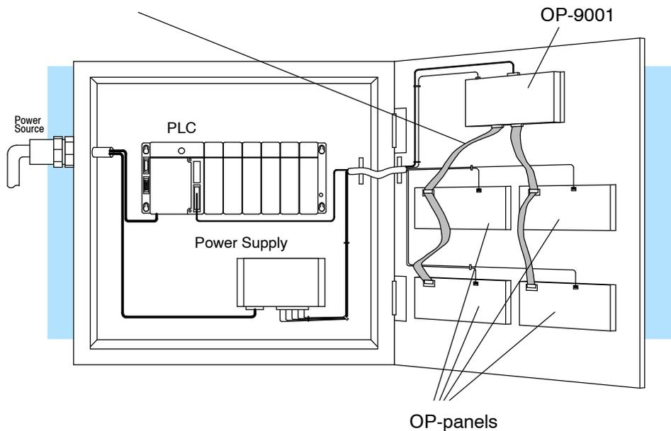
**Note:** Panels can be located as far away as 4000 feet from the OP-9001 when using shielded cable (Belden 9729 or equivalent). Flat ribbon connections can be used for a distance of 30 feet maximum. For ribbon cable, we recommend Belden 9L28015 or 3M 3365/15.
