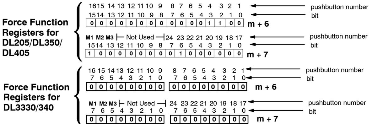
Think of forcing as a one-shot process. That is, once you have set the mode in m+7, the bit patterns in m and m+1 are changed (according to the mode selected), and then, all of the bits in m+6 and m+7 are set to zero. What this means is that all pushbuttons return to normal manual operation after the forcing is completed.
