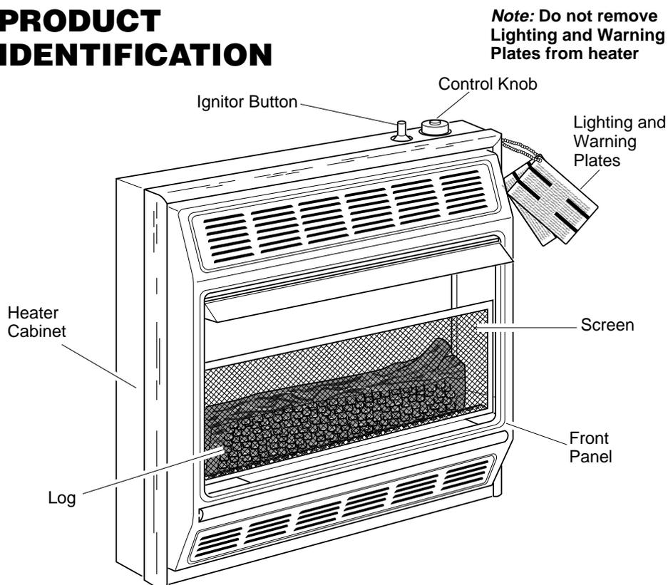
Figure 1 - Vent-Free Gas Log Natural Gas Space Heater
