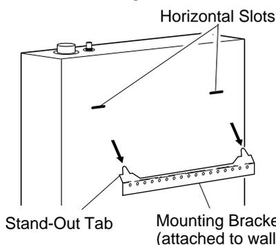
Figure 14 - Mounting Heater Onto Mounting Bracket
