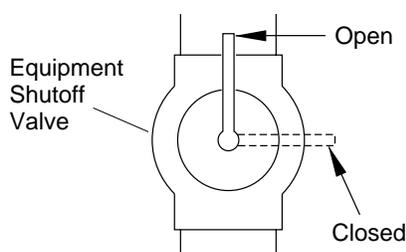
**Figure 19 - Equipment Shutoff Valve**
