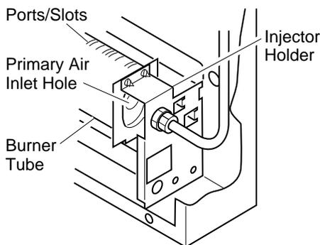
**Figure 27 - Injector Holder On Outlet Burner Tube**
