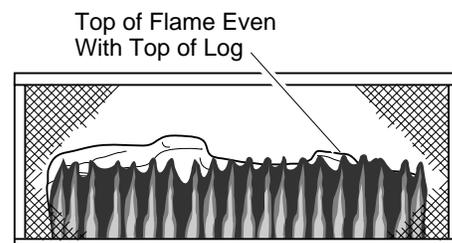
Figure 25 - Correct Burner Flame Pattern
