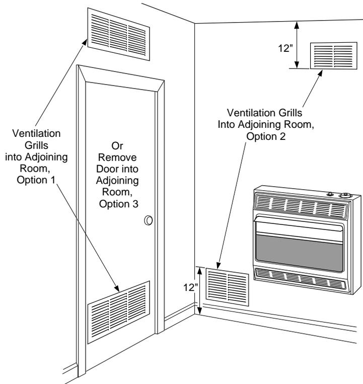
Figure 7 - Ventilation Air from Inside Building
