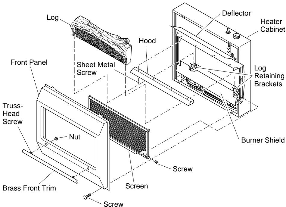
**Figure 3 - Assembling Heater**
