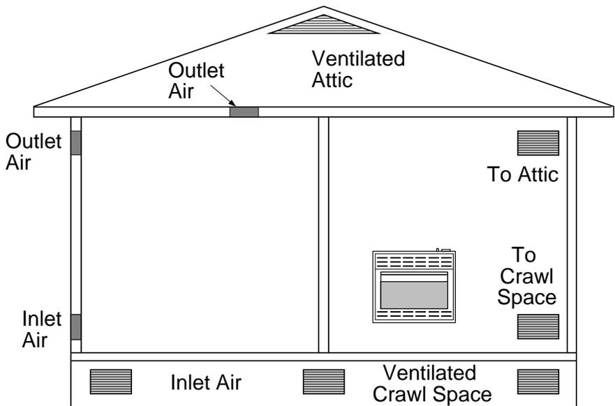
Figure 8 - Ventilation Air from Outdoors
