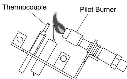
Figure 24 - Incorrect Pilot Flame Pattern
