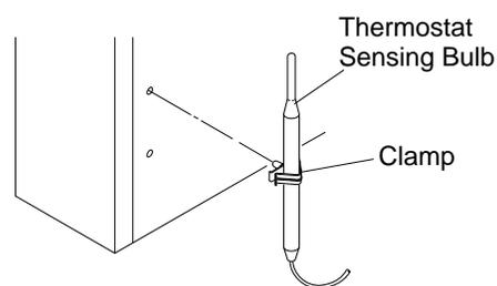
**Figure 10 - Attaching Thermostat Sensing Bulb**
