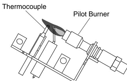
Figure 23 - Correct Pilot Flame Pattern
