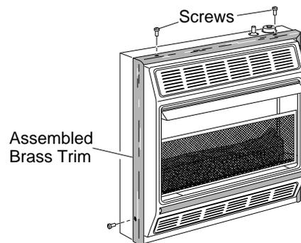
**Figure 6 - Attaching Brass Trim to Heater**
