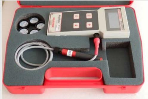
The sensitive region of the probe is indicated by the red disc at the probe end.
