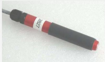
number standards prepared by the National Institute of Standards and Technologies (NIST) in USA. Sixteen standards are used ranging from 0.5 to 111.9 FN giving an instrument with a measurement range from 0 to 115 FN. Transfer standards are supplied with the instrument allowing performance to be verified at any time.
