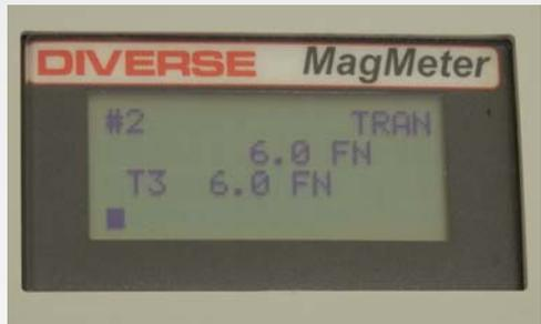
To cycle through the transfer standards use the ▲ up or ▼ down keys. This mode facilitates checking the veracity of the instrument.
