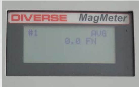
There are 52 available records and the current measurement value can be saved by pressing the ⓘ power key. The oldest record is overwritten.
