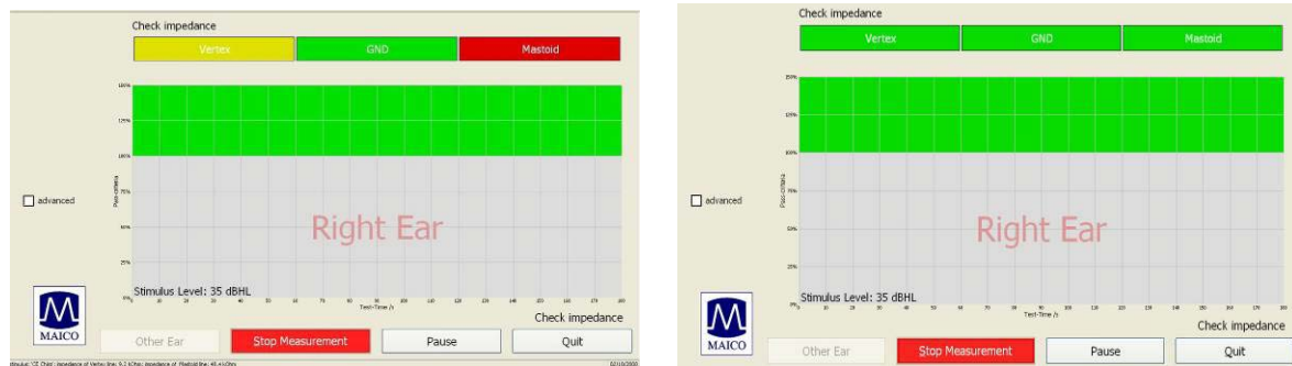
Figure 17 Impedance traffic lights at top of measurement window
