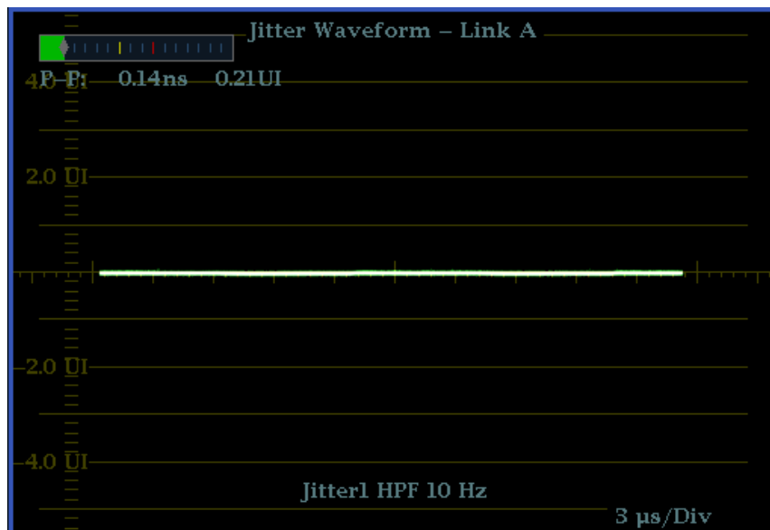
Figure 32: The Jitter display parameters as shown in a single tile when the instrument is in 4-tile mode
