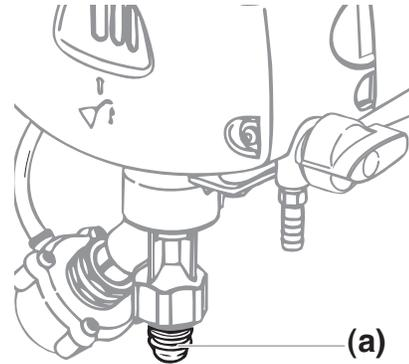
3. When suction set is clean, thread the suction tube back into the inlet valve, and replace the return tube onto the return tube fitting. Replace clip.
