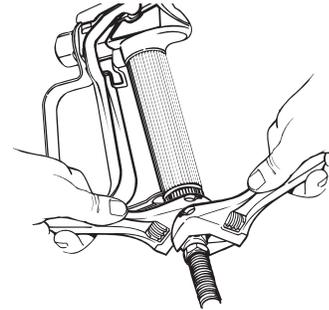
3. Remove filter from spray gun (refer to [Cleaning the Spray Gun Filter](#), page 12).
