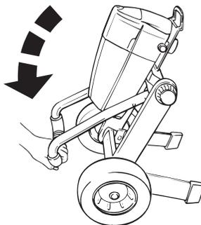
3. Lift the leg lock, and fold the legs in. Replace the leg lock to hold the legs into place (inset).
