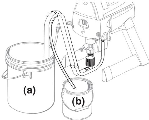
4. Slide the PressureTrac™ to maximum pressure (+). Turn the PRIME/SPRAY knob to PRIME.
