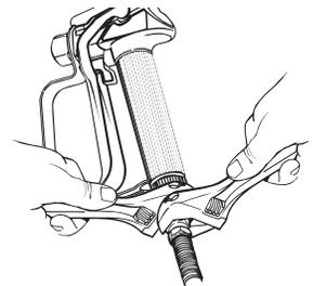
6. Remove cap from inlet valve (a). Thread the suction tube onto the inlet valve and tighten firmly by hand. Be sure that the threads are straight so that the fitting turns freely.
