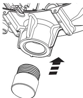
4. Install the new O-ring on the inlet valve assembly, lubricate with Separating Oil (P/N 0516444, sold separately) or light household oil, thread into the bottom (inlet) of the housing, and tighten with an adjustable wrench. This will drive the bottom seal into the correct position.
