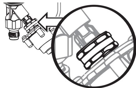
If priming problems persist, you may need to replace the inlet valve assembly. Call Technical Service to order new inlet valve assembly.
