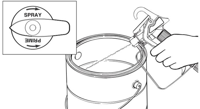
4. Release trigger. Turn the PRIME/SPRAY knob to PRIME. Turn the pump OFF (O). Trigger the gun into the waste container to be sure that no pressure is left in the hose.
