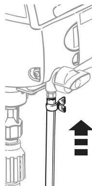
8. Verify that the seal is present inside the suction tube. Thread the inlet filter into the end of the suction tube.
