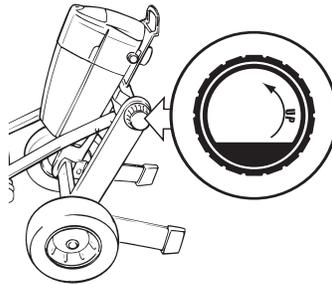
3. Lift the handle until the motor housing and handle locks into place. **Be careful not to pinch the power cord with the cart.**
