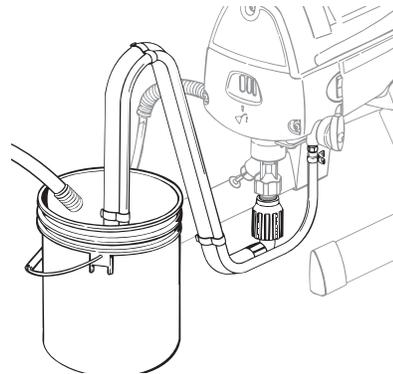
3. Remove the inlet filter from the suction tube and place into the waste container.
