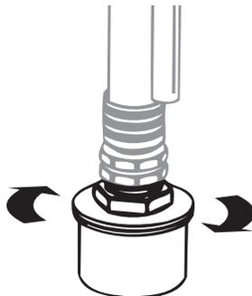
4. Verify that the seals are present inside the adapter and suction tube (a). Thread the pump cleaning adapter (b) onto a garden hose (c). Connect hose and adapter to the fitting on the end of the suction tube (d).
