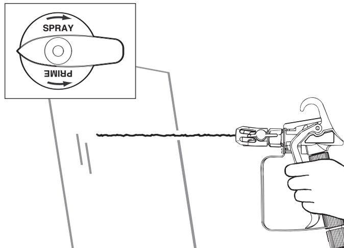
4. Release the trigger and lock the gun off (see page 7).
