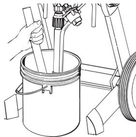
2. Turn the PRIME/SPRAY knob to PRIME. Plug sprayer in. Turn the switch to ON (I).
