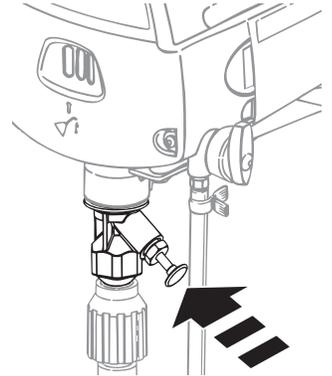
3. Place a full container of spraying material underneath the suction tube (a). Secure the return tube (b) into a waste container.
