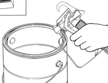
6. Let the pump circulate cleaning solution through the suction set for 2-3 minutes. Turn the pump OFF.
