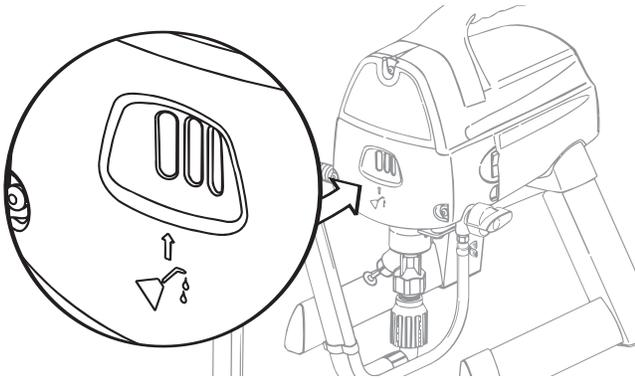
2. If you have a model XT250, fully insert the Quickflo™ valve to make sure the inlet ball is free.
