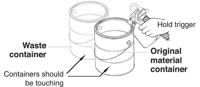
3. While pulling the gun trigger, turn the pump ON (I), and turn the PRIME/ SPRAY knob to SPRAY to purge material from the hose back into the original container.
