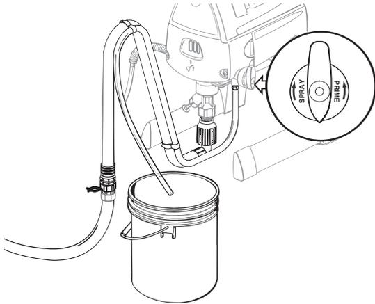
6. Turn water supply on. Turn pump ON (I). Water will go into the suction tube and out through the return tube. Let pump run for a few minutes to allow the return tube to be flushed.
