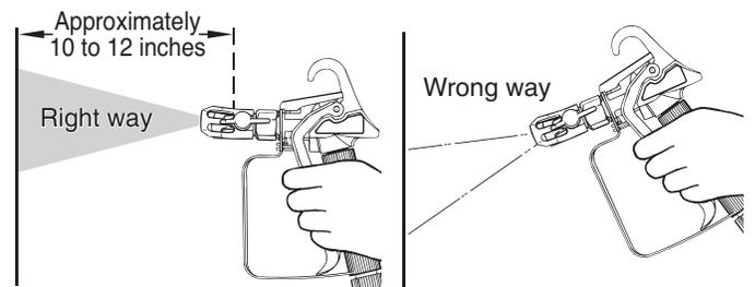
**Tip:** Trigger gun after starting the stroke. Release the trigger before ending the stroke. The spray gun should be moving when the trigger is pulled and released. **Overlap each stroke by about 30%. This will ensure an even coating.**
