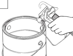
5. Lock the spray gun off. Thread the spray tip guard assembly onto the gun. Tighten by hand.
