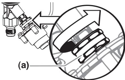
2. Unscrew the **inlet valve assembly (b)** from the sprayer. Visually inspect the inside and outside of the inlet valve assembly. Clean any paint residue with the appropriate cleaning solution.
