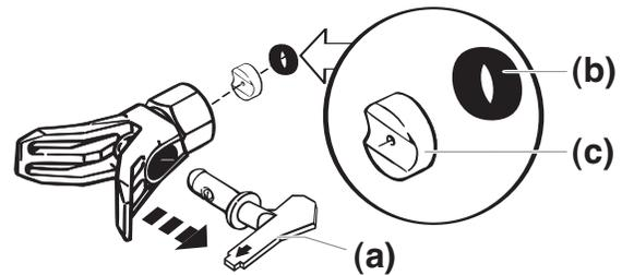
5. Install gun filter tapered-end first. Reassemble spray gun.
