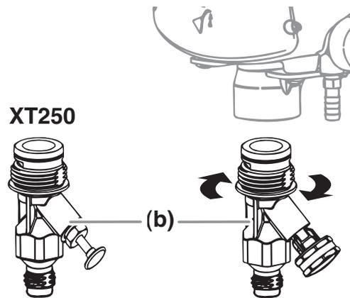
3. Replace inlet valve assembly by screwing it into the sprayer.
