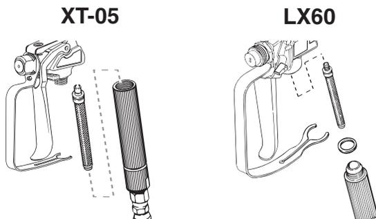
6. Install spray tip (a), saddle seat (c) and washer (b), and replace spray guard assembly.
