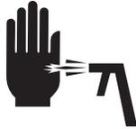
**DO NOT TREAT AN INJECTION INJURY AS A SIMPLE CUT!** Injection can lead to amputation. See a physician immediately.
