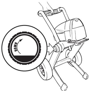
2. When the knob is fully "DOWN", this will release the handle and it can be folded down until it is locked into place. **Be careful not to pinch the power cord with the cart.**
