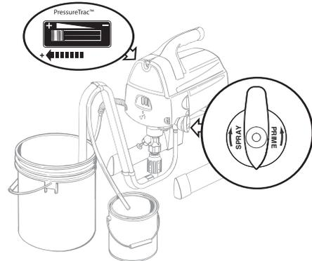
5. Plug in the sprayer and move the ON/OFF switch to the ON (I) position.
