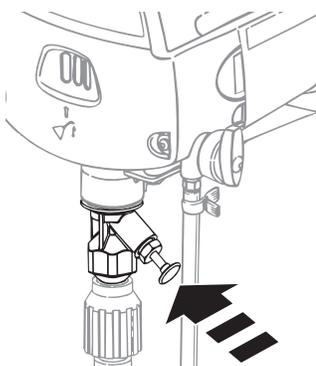
4. Wipe the entire unit, hose and gun with a damp cloth to remove accumulated paint. Replace the high pressure hose to the paint hose port.
