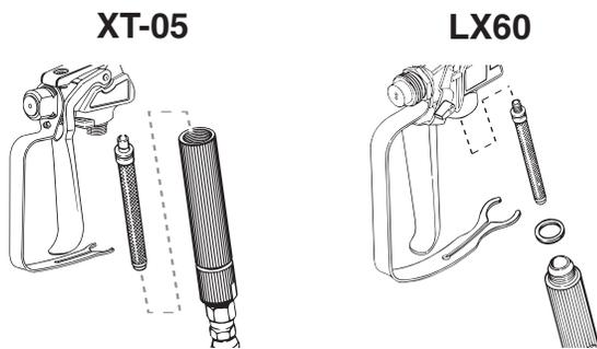
4. Remove spray tip (a) from spray guard assembly. Clean spray tip with a soft-bristled brush and the appropriate cleaning solution. Be sure to remove and clean the washer (b) and saddle seat (c) located in the rear of the spray tip assembly.
