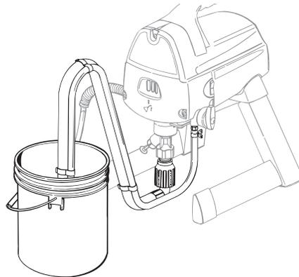
5. Turn the PRIME/SPRAY knob to PRIME. Turn the pump ON (I), and trigger the gun **once** into a waste container to relieve pressure.
