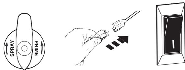
3. Turn the PRIME/SPRAY knob to SPRAY. Test the sprayer on a practice piece and begin spraying.
