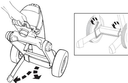
2. Twist the knob on either side of the cart toward the "UP" arrow until it stops.
