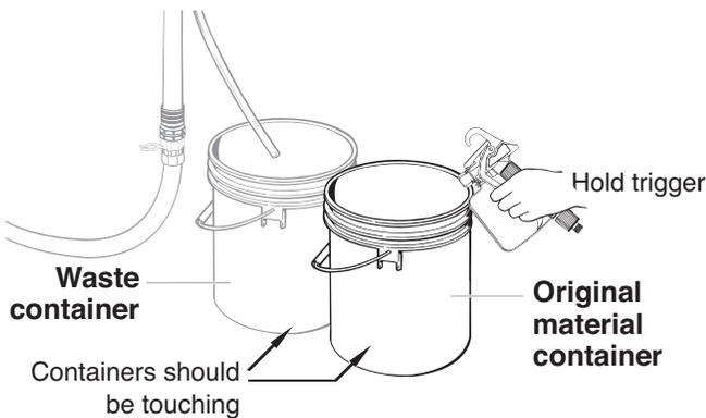
8. While pulling the trigger, turn the PRIME/SPRAY knob to SPRAY to purge material from the hose back into the original container.
