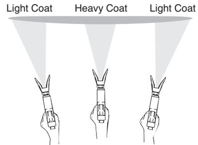
**Tip:** Keep the spray gun perpendicular to the surface, otherwise one end of the pattern will be thicker than the other.
