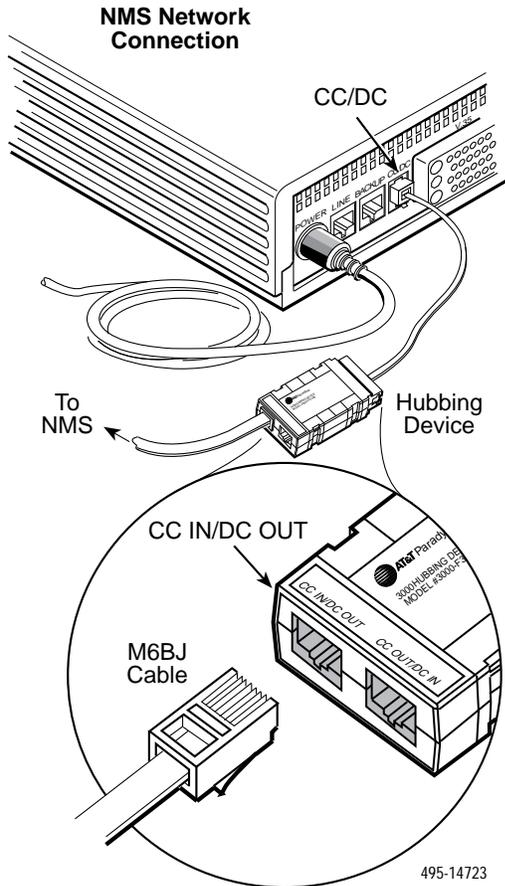
2. Plug one end of the 6-pin cable into the hubbing device jack labeled **CC IN/DC OUT**.
