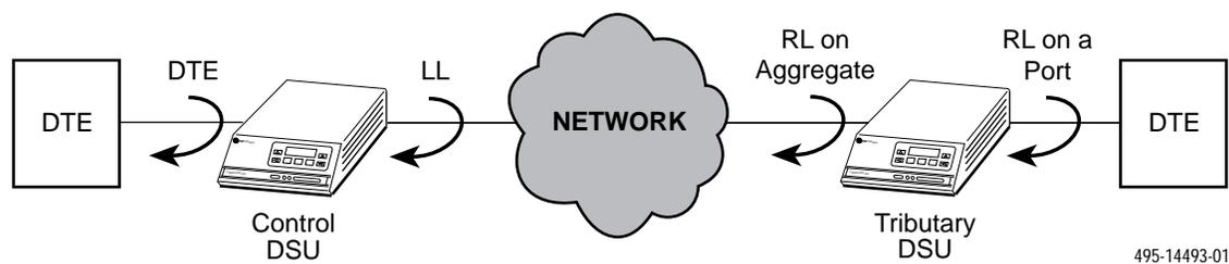
Figure 3-3. Loopbacks, Example 1
