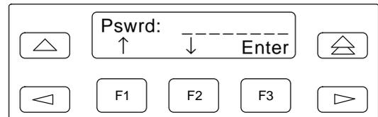
5. Enter the previously configured password and press **F3**. The async terminal is now enabled and the front panel is disabled (locked). The LCD displays **User I/F – Idle**.
