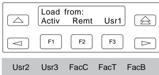
4. The selections on the screen are configuration option sets stored in the DSU's memory. Table 2-1 lists the **Load from** menu selections and their source.
