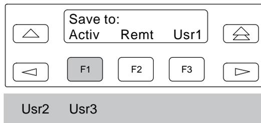
When you select from the **Save to** screen, the DSU performs a verification routine to ensure that the configuration options chosen are compatible.
