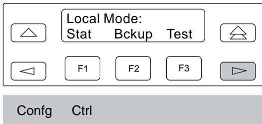
2. To access the Configuration (**Config**) branch, press the **▶** key until **Config** appears. Press the function key below **Config**. The following screen appears.
