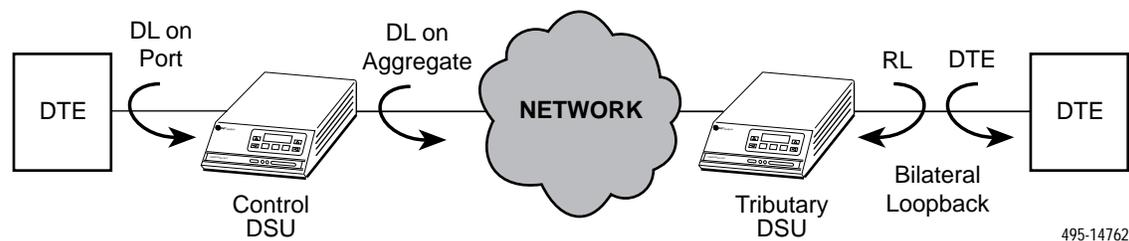
Figure 3-4. Loopbacks, Example 2
