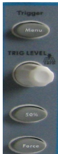
Fig.4-14 Trigger Control Zone
