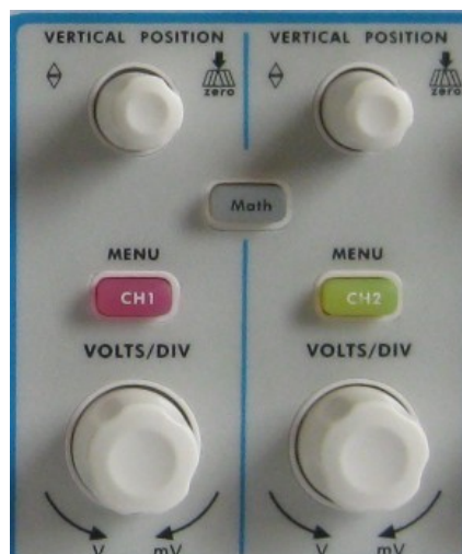
Fig. 4-12 Vertical Control Zone
