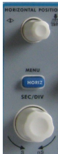
Fig. 4-13 Horizontal Control Zone
