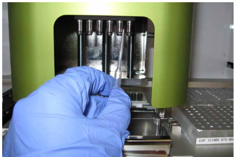
Figure 3.17 Lubricating the O-rings
