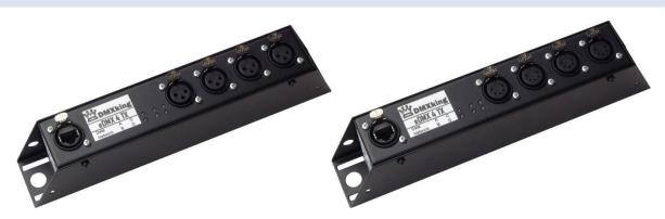
Ethercon connector for power/network using 802.3af PoE switch or power injector. Higher power 802.3at switches/injectors will also work. Four female 3pin or 5pin XLR connectors for DMX512-A *input (eDMX4 RDM only)* or *output* function on each port.
