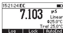
**Non Linear Temperature Compensation:** for natural water measurements.
