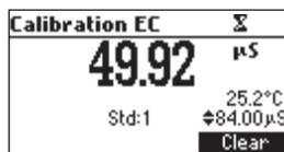
All old calibrations will then be cleared and the instrument continues calibration. The points confirmed in current calibration are kept.
