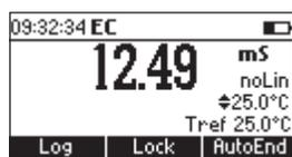
The conductivity of natural water shows strong non-linear temperature behavior. A polynomial relationship is used to improve the accuracy of the calculated results.
