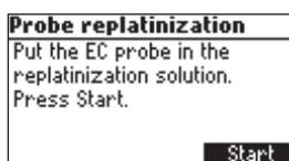
Put the probe into a beaker with replatinization solution and press **Start**.
