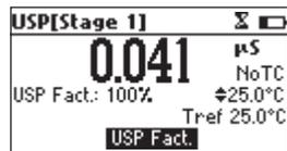
If the temperature source is manual entry, press **USP Fact.** to select USP factor to be changed (the  $\diamond$  is displayed before the 100% value). To increase the accuracy of the analysis decrease the USP factor value.
