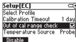
Press the corresponding functional key in order to enable/disable this feature. If enabled, a warning message is displayed when the EC reading is too far from the EC calibration points.
