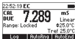
The calibration time out can be set (see SETUP for details, page 35) from 1 to 7 days or can be disabled.
