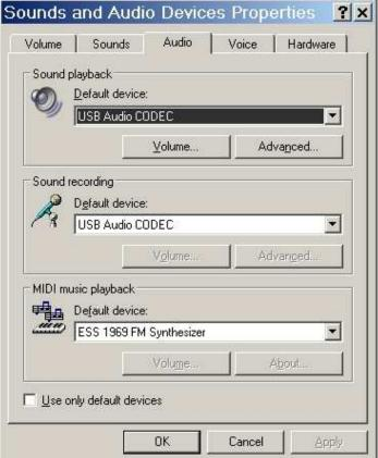
In Windows 2000 and Windows XP, open "Sounds and Audio Devices" in the Control Panel or right click on the Speaker icon on the Taskbar and select Adjust Audio Properties. Reset the Default device for Sound Playback and Sound Recording to your computer's primary sound device.
