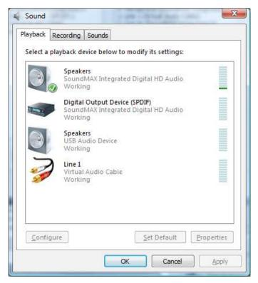
Windows will automatically install the USB Audio Device driver to support the USB Audio CODEC in USB Interface III.
