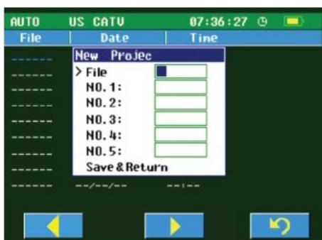
The unit will show the list of files in storage. Using **UP/DOWN** arrow key select an empty file and
