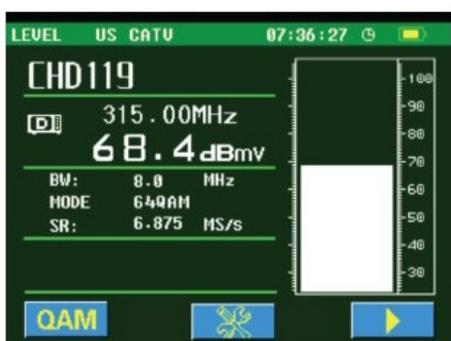
Press **UP/DOWN** or **LEFT/RIGHT** arrow key to change the testing channel.
