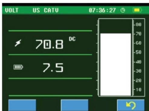
In the main menu, using the **LEFT/RIGHT** key highlight the icon “VOLTAGE” and press the **CH/ENTER** key, the meter enters the voltage measurement mode.
