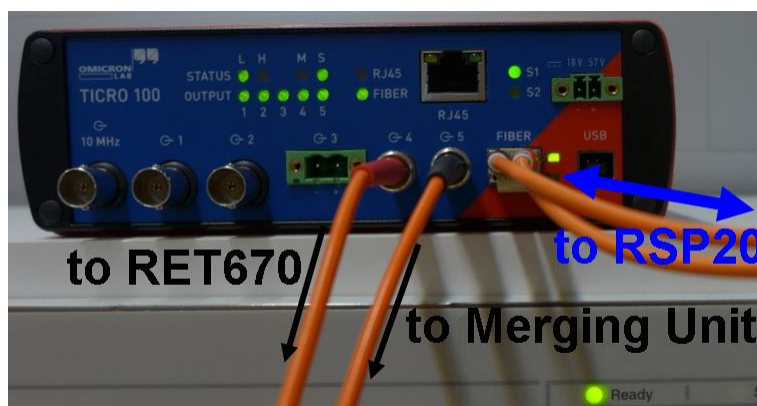
Figure 2: Connecting RET670 with TICRO 100
