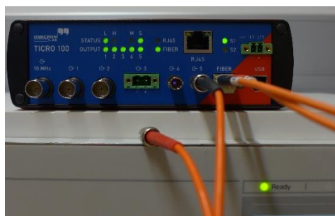
Figure 14: red IRIG-B ST Fiber disconnected
