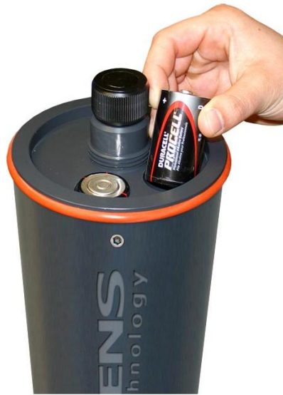
Figure 3: Installing batteries in the SDL500
