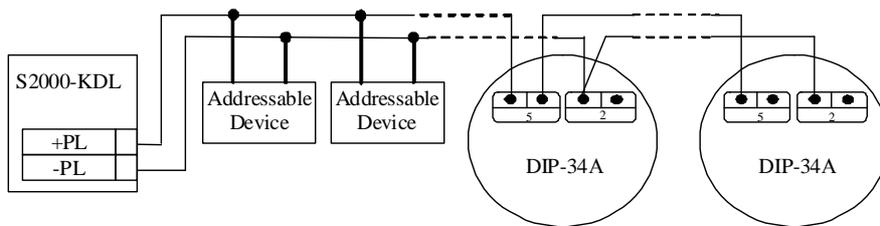
Figure 3. Wiring Diagram
