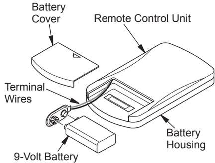
Figure 24 - Installing Battery in Hand-Held Remote Control Unit
