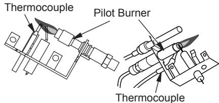
**Figure 36 - Correct Pilot Flame Pattern**
