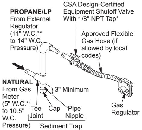
**Figure 15 - Gas Connection (Thermostatically-Controlled Models Only)**
