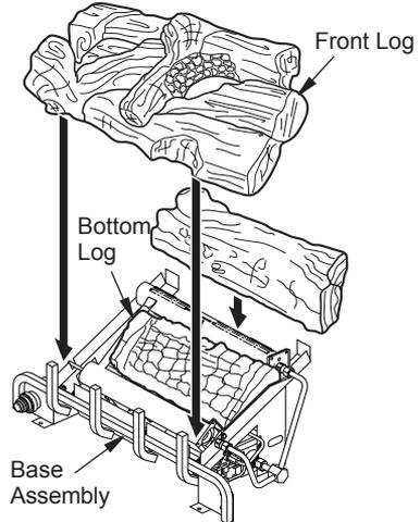
**Figure 27 - Installing CRB and HRB Model Log Sets**
