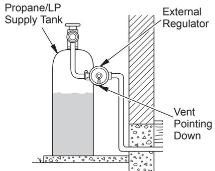
**Figure 14 - External Regulator With Vent Pointing Down**
