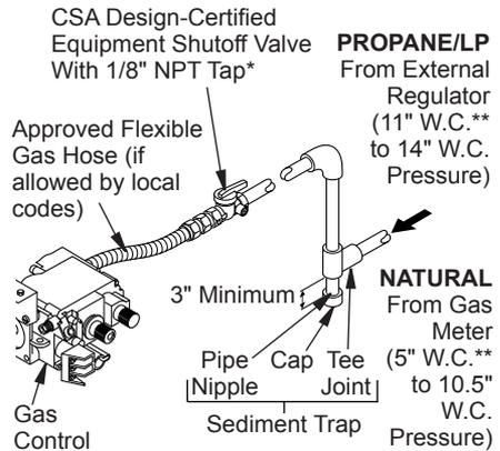
**Figure 16 - Gas Connection (Remote-Ready Models Only)**
