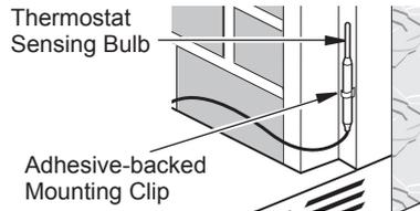
**Figure 46 - Locating Thermostat Sensing Bulb on Factory-built Metal Fireplace**
