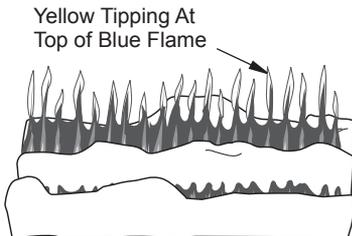
**Figure 39 - Incorrect Front Burner Flame Pattern**
