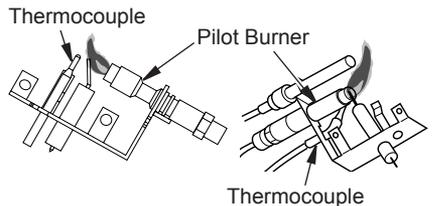
**Figure 37 - Incorrect Pilot Flame Pattern**
