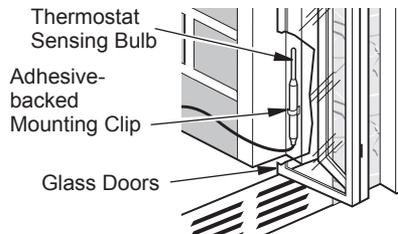
**Figure 47 - Installing Thermostat Sensing Bulb Behind Glass Doors**
