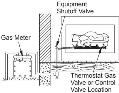
**Figure 19 - Checking Gas Joints (Natural Gas Only)**
