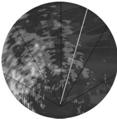
**WX NORM** - Selects the normal condition of operation for weather detection. The system will transmit after a 60 second warm-up time is completed. The radar system initializes to the Wx mode, 50 nm.
