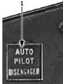
A red light marked AUTOPILOT DISENGAGED is on both the Captain's and the First Officer's panel. With the autopilot engaged, the lights will come on flashing any time either or both channels of the autopilot become disengaged for any reason.
