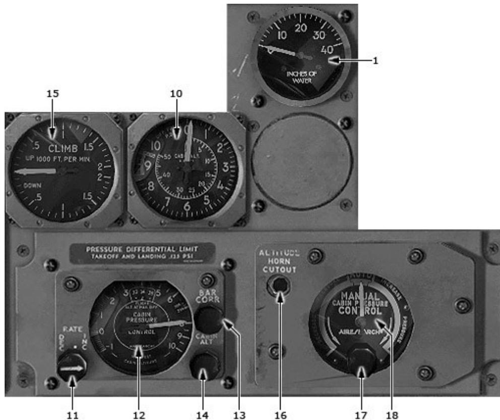
1. Conditioned Air Duct Pressure Indicator
