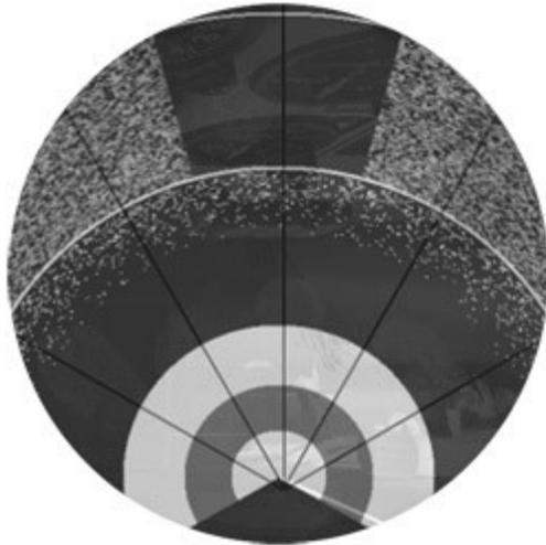
**TEST** – Transmitter de-energized. contrasting test signals are imposed on the indicator, signifying proper circuit functions.
