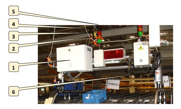
**1. POWER ON INDICATOR LIGHT:** If the controller is on, the "POWER" labeled light glows.
