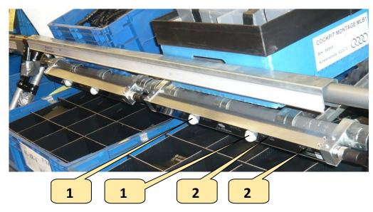
The light curtains are designed for 300mm, 400mm and 600mm storage boxes.
