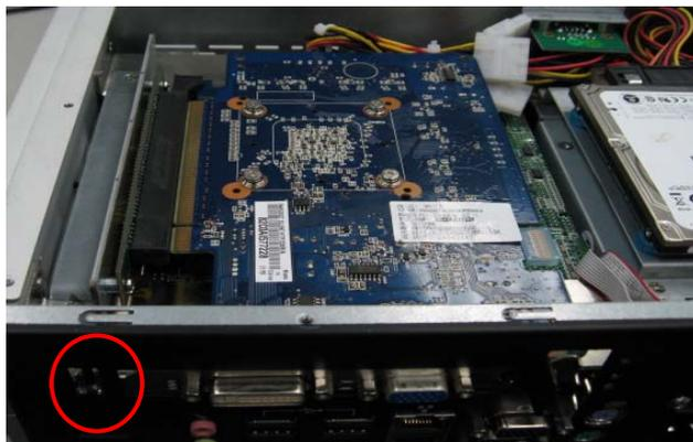
**Step 6** Once the card is seated in the slot, screw the bracket onto the rear panel.
