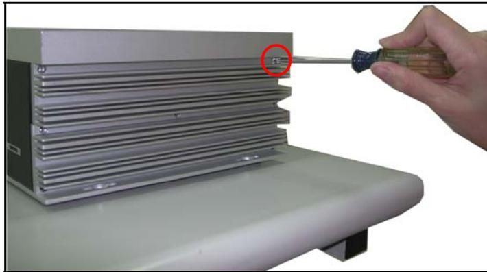
**Step 4** Remove the cover from the chassis.
