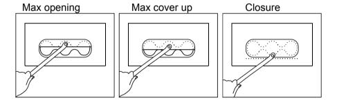
Closing the reservoir shutter completely will cause the flame to be extinguished.
