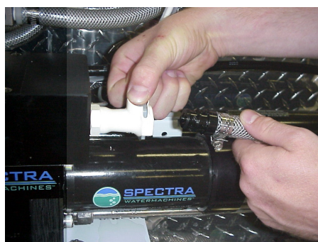
Attaching brine discharge service hose
