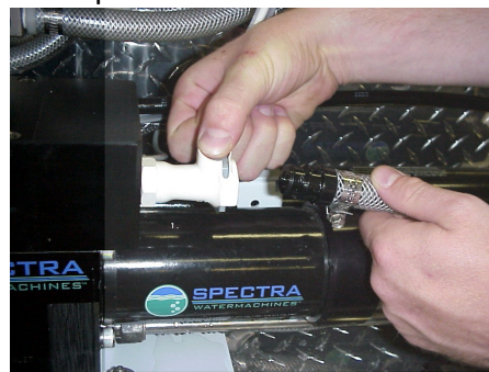
Connecting brine discharge service-hose
