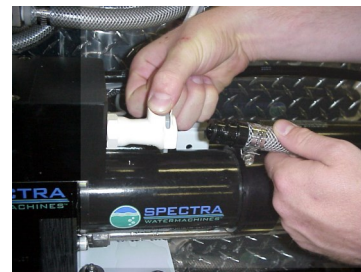
Connecting brine discharge service hose
