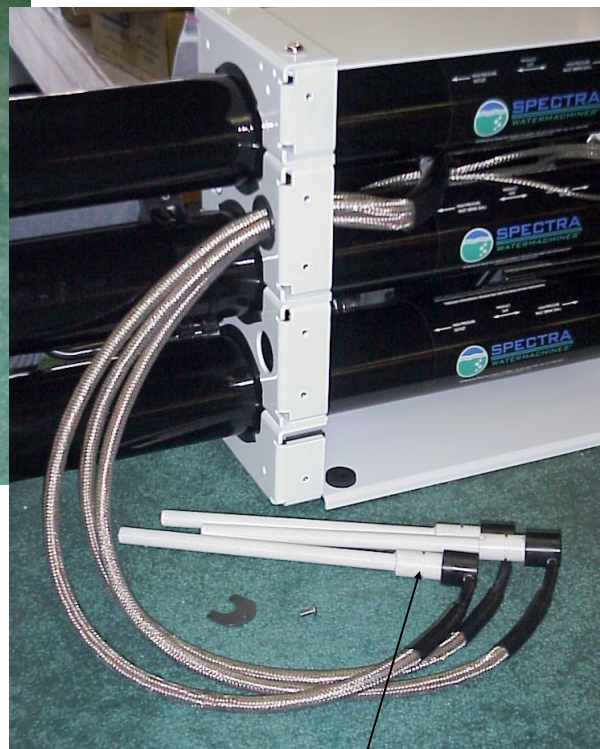
C-Clip groove in Anode
