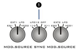
Oscillator sync is where the master signal will reset the waveform of the slave signal each time the master waveform starts a new cycle.
