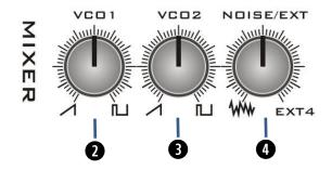
**NOISE GENERATOR:** The noise generator produces white noise. This is like the hiss you hear between radio stations. The signal is available for filtering via the Noise/EXT4 mixer control.
