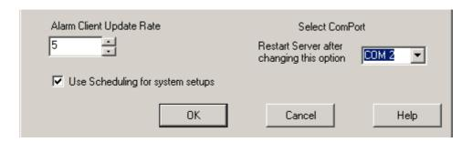
Use the 'Select ComPort' spin box to chose a valid RS232 com port for the Server PC to communicate with an attached E-Series frame or linked-frame system.
