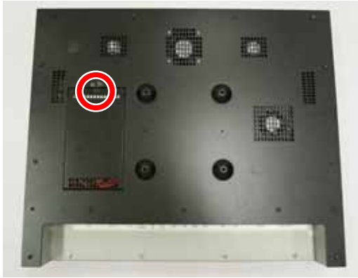
a. Loosen the screw (1) on the HDD Door
