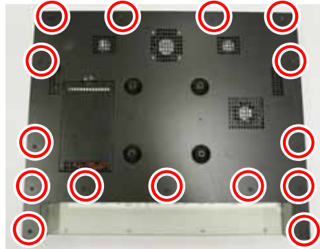
b. Loosen the screw (15) on the rear cover
