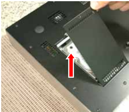
a. Disconnect HDD Cable (Refer to Chapter 4.1)
