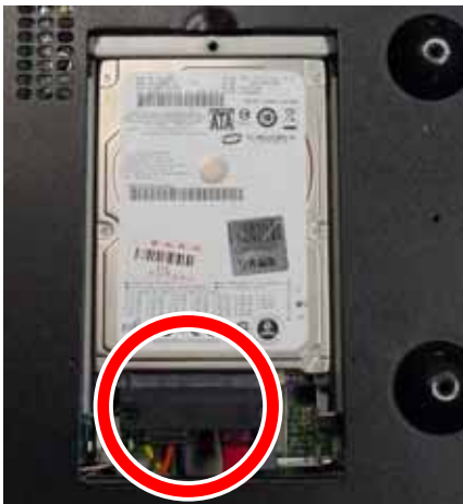
c. Disconnect the Cable (1) to replace the HDD
