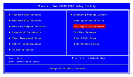
This option is for setting a password for entering BIOS Setup. When a password has been set, a password prompt will be displayed whenever BIOS Setup is run. This prevents an unauthorized person from changing any part of your system configuration.
