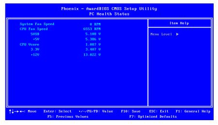
The PC Health Status displays the current status of all of the monitored hardware devices/components such as CPU voltages, temperatures and fan speeds.
