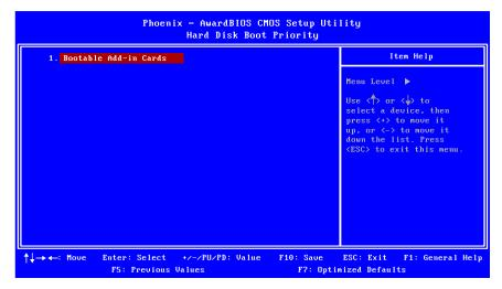
This is for setting the priority of the hard disk boot order when the "Hard Disk" option is selected in the "[First/Second/Third] Boot Device" menu item.
