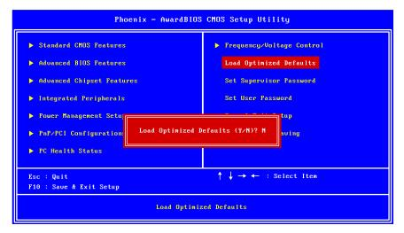
This option is for restoring all the default optimized BIOS settings. The default optimized values are set by the mainboard manufacturer to provide a stable system with optimized performance. Entering "Y" and press < Enter> to load the default optimized BIOS values. Entering "N" will cancel the load optimized defaults request.
