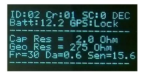
The Boom Box 3 has a graphical display. The display is used to show the setup of the box at power on, the CAP and Geophone resistance, the ready message, the uphole information, and the shot status message. The display shows the following messages:
