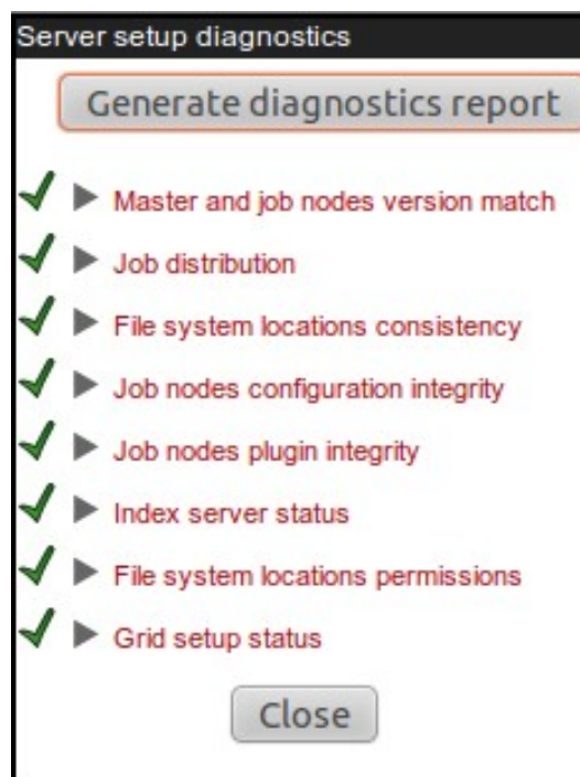
Figure B.1: Check system. Failed elements will be marked with a red X. If you have not configured your Server to submit jobs to a local Grid system, or if you have and your setup is configured correctly, you will see a green checkmark beside the Grid setup status item in the diagnostic report.
