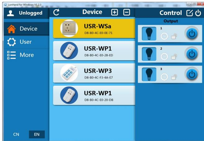
The control menu displays the control button, which is close by default. You can click the button to control switch as shown in the diagram. Also the button will change accordingly to the switch state.
