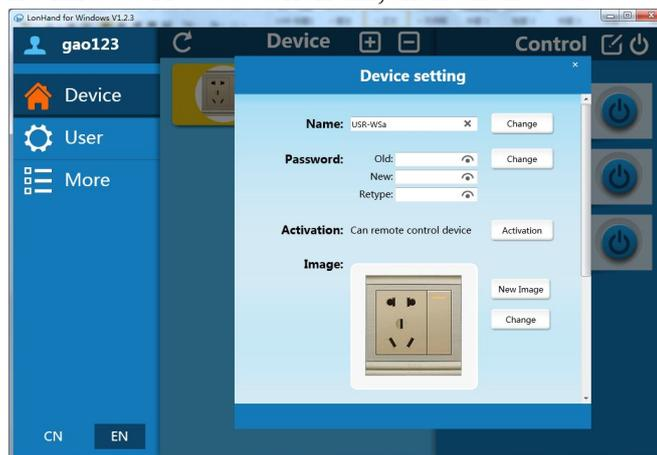
Change you network or you control it remotely, click “Synchronized to local”, refresh the device list, you will see the device icon into a remote icon, then you can control the devices via internet.
