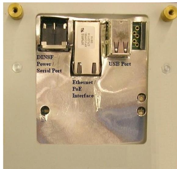
Figure 3—Connector Location—Rear of ScanVue®
