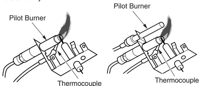
**Figure 43 - Incorrect Pilot Flame Pattern (Your pilot may vary from pilots shown)**
