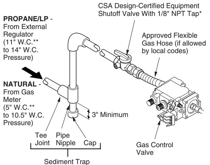
**Figure 15 - Gas Connection (Remote-Ready Models Only)**
