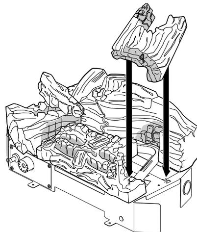
Figure 31 - Installing Log #4 (Model LGX3924NT Shown)
