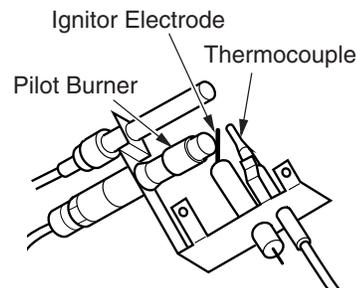
Figure 38 - Pilot (Propane/LP) Figure 39 - Pilot (Natural)
