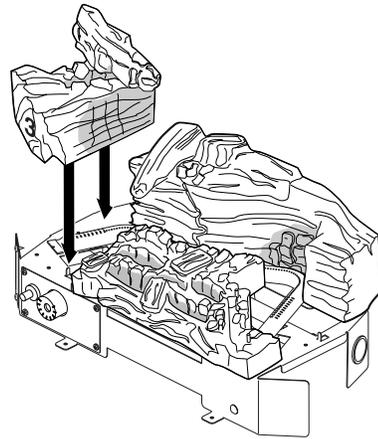
Figure 30 - Installing Log #3 (Model LGX3924NT Shown)
