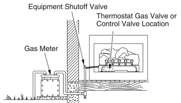
**Figure 18 - Checking Gas Joints (Natural Gas only)**
