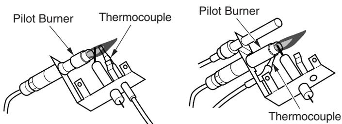
**Figure 42 - Correct Pilot Flame Pattern (Your pilot may vary from pilots shown)**
