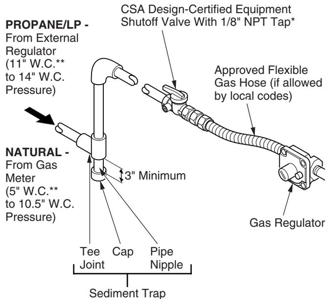
**Figure 14 - Gas Connection (Thermostat-Controlled Models Only)**
