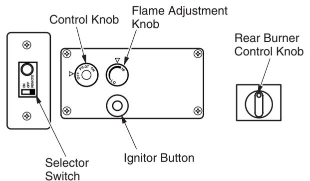
**Figure 40 - Control Knobs, Selector Switch and Ignitor Button Locations for Remote Operation**
