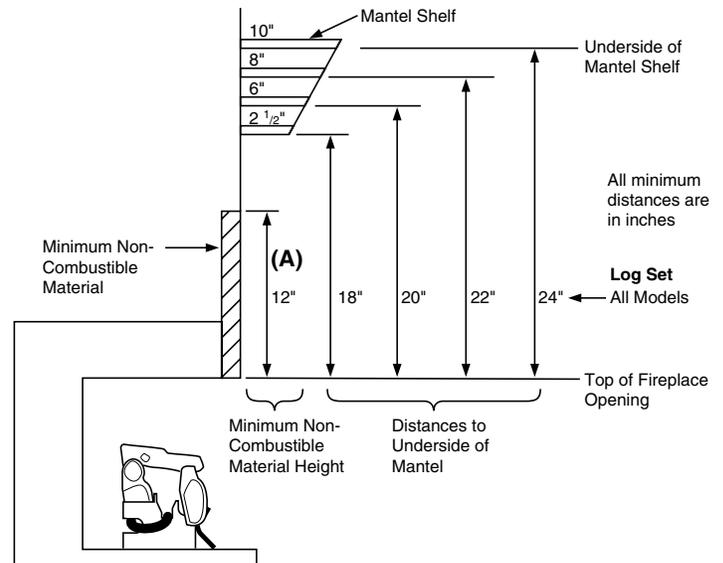
Figure 6 - Minimum Mantel Clearances Without Using Hood
