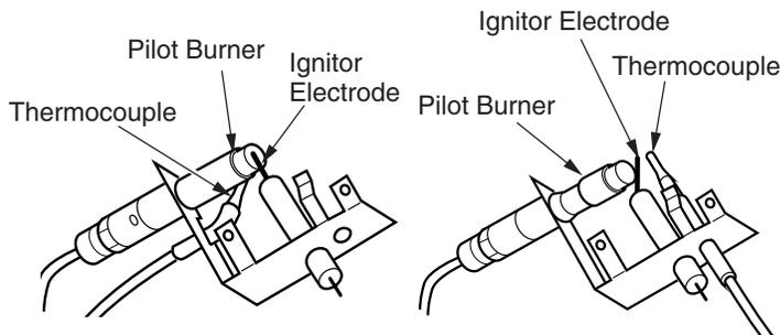
Figure 35 - Pilot (Propane/LP) Figure 36 - Pilot (Natural)
