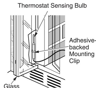
**Figure 53 - Installing Thermostat Sensing Bulb behind Glass Doors**
