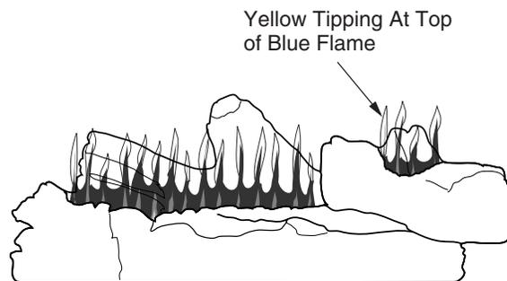
**Figure 45 - Incorrect Front Burner Flame Pattern**
