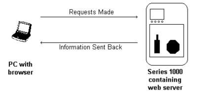
Each Series 1000 with Aztec On-line<sup>™</sup> has a unique telephone number. To view pages stored by the Series 1000, dial the telephone number of the monitor and enter a predefined IP address in your browser. The pages displayed will give you information about the Series 1000 and let you control its operation.
