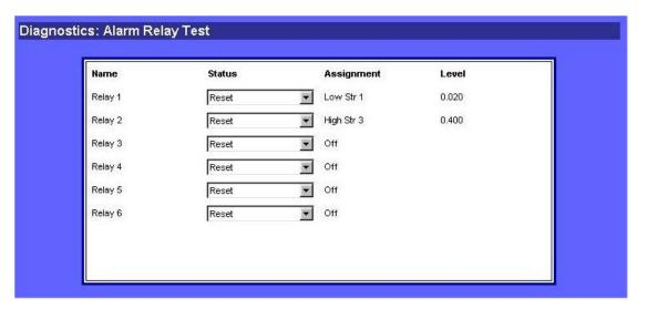
You must be logged in with full security rights (Level 3) to perform an alarm relay test.
