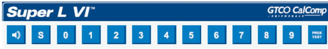
The SuperSet Menu is used to prepare the digitizer to receive specific, detailed custom configuration information from the Tablet Configuration Utilities for some serial installations. Use your transducer (pen or cursor) to click on the menu buttons to make your selections.
