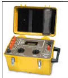
The Digital Ground Resistance Tester Model 4500 is designed for measuring very low resistance on large grounding systems, such as ground grids and ground mats. It rejects high levels of interference voltages at DC or 60 Hz and its harmonics, and can be used under difficult conditions such as high stray current or excessive auxiliary electrode resistance.
