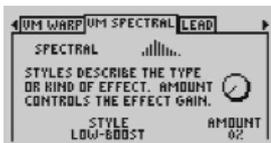
\* Special Note: Each VM effect menu has an *AMOUNT* control to 'dial in' the amount of effect desired. Remember that there is also a *DRY:VM MIX* control in the LEAD menu that determines how much of the input vocal is left Dry and how much is passed through VM. The setting of this ratio can determine the effectiveness of your other parameter settings, as it is essentially a master mix control for the Dry and VM Lead voice.
