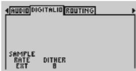
*DITHERING* can be set to 8, 16 or 20 bits, or an '*OFF*' position.
