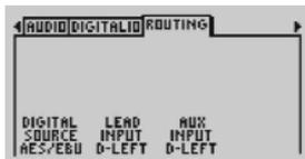
*LEAD INPUT*: to use your analog line in on the back panel, or the Mic preamp on the front of your VoicePrism Plus, set the *LEAD INPUT* to ANALOG. To use the microphone input, the **MIC ON** button must be selected, as well as
