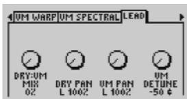
DRY:VM MIX (0-100% MODELED): sets the balance between the Dry Lead voice, and the VM Lead voice. 100% is undiluted VM voice, and 0% is Dry voice.
