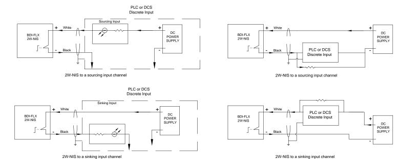
**Note:** The shield (drain wire) of the 2W-NIS output cable should be connected to ground at the PLC or DCS site and ground only at one point throughout the shield.
