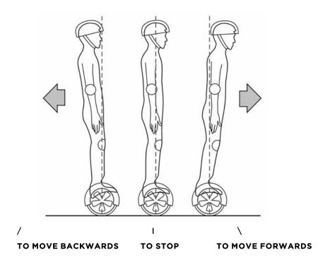
Notice in the diagram above, your center of gravity determines which direction you move, accelerate, decelerate, and come to a complete stop.
