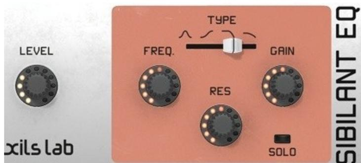
Select your filter type from **Low-pass 6dB**, **Low-Pass 12 dB**, **Bell** or **High-shelf** by clicking on the corresponding button. Adjust the Cut-off frequency with the **FREQ** knob, the Resonance (or emphasis) with the **RES** knob and for the Bell and the Shelf filter, the gain with the **GAIN** knob.
