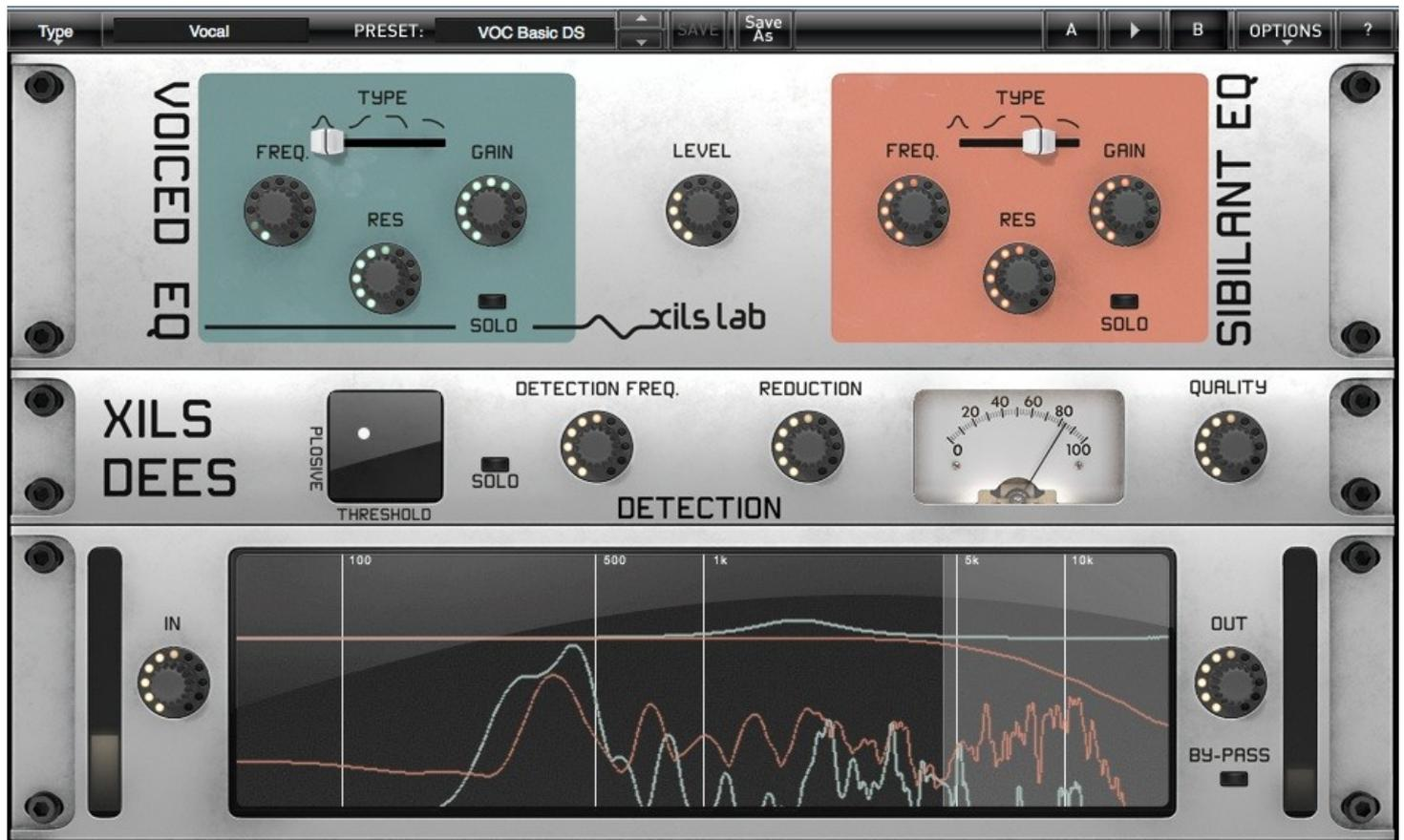
From this default settings, click on **SOLO** under the reduction vu-meter, tweak the frequency knob to adjust the cut-off frequency of the high pass filter which removes low ends from the detection path.
