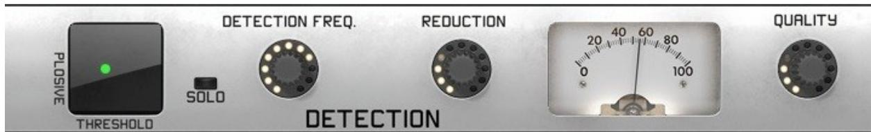
The detection begins with a High Pass filter to remove the low end of the input signal from the detection path. The cutoff frequency of this filter is adjusted with the **FREQUENCY** knob and the result can be listened to by clicking on the **SOLO** button. This filter helps to isolate the sibilant from the voiced part.
