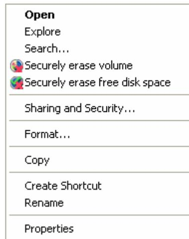
Figure 4 Context Menu for the Secure Deletion of Free Disk Space
