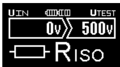
Fig. 3.5 Example of setting for insulation resistance measurement
