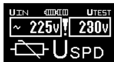
Fig. 3.4b Example of voltage measurement (USPD function)
