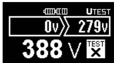
Fig. 3.10b Another example of USPD measurement result (discharged)
