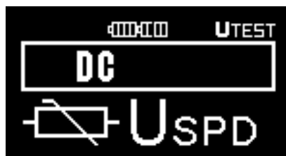
Fig. 3.8 Example of setting of SPD function, DC function selected
