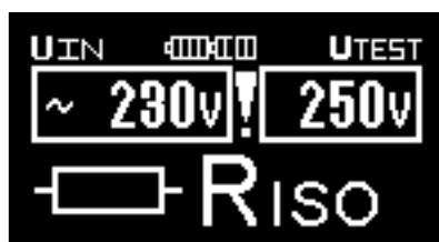
Fig. 3.4a Example of voltage measurement (RISO function)
